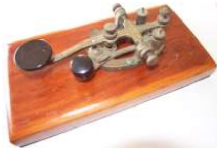
U.S. style key (The box label read 'HAND TELEGRAPH KEY U.S. NAVY TYPE 26001-B Made by BUZZA PRODUCTS, SYDNEY')
